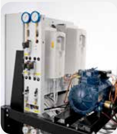
Pannello pressostati BT e inverter TN/BT. Pressure switch panel and frequency inverter MT/LT.
